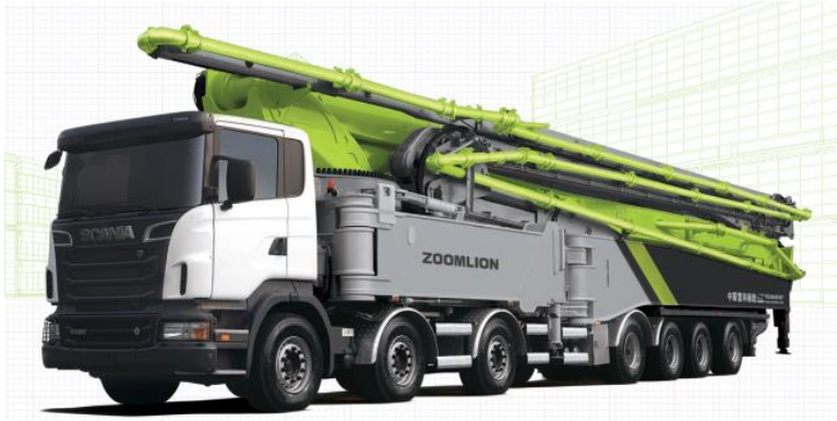
Gambar 2.17 Concrete Pump Zoomlion 43X-5RZ Sumber: Brosur Zoomlion (2016)
