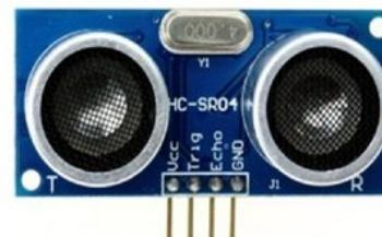
Gambar 4. Sensor jarak *ultrasonic HC-SR04*
