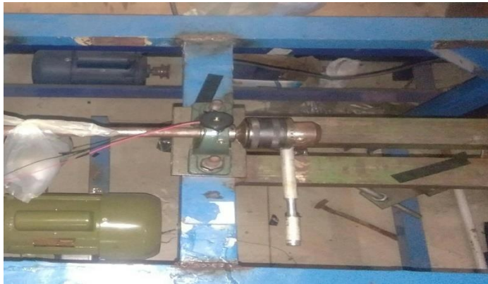
Gambar 2. Sensor getar diatas bearing .
