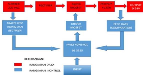
Gambar 6. Blok Diagram power supply switching
