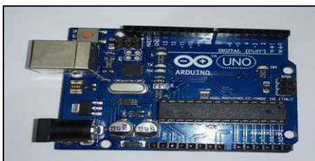
Gambar 2. 2 Papan Arduino (Sumber: Abdul Kadir, 2017)
