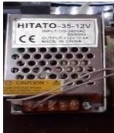
Gambar 4. 13 Power Supply 12V 3A
