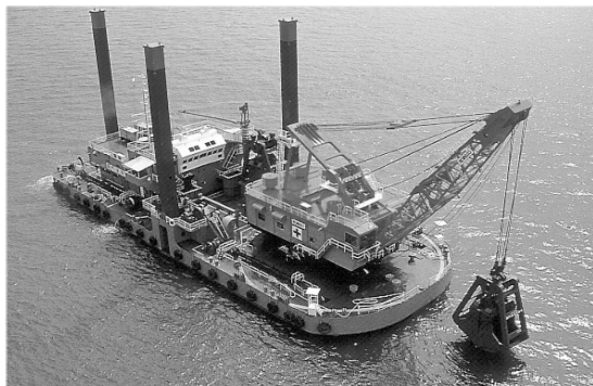
Gambar 2.2. Grab or Clamshell Dredger
