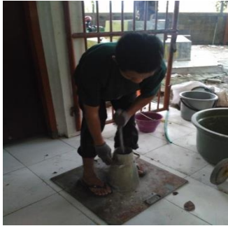
Proses Slump Test
