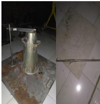
Alat Slump test
