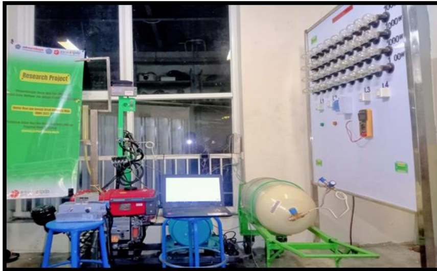
Figure 2. Laboratory-Scale Prototype of Natural Gas/Diesel Dual Fuel System with HHO Injection
