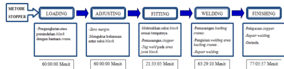
Gambar 3. Diagram Value Stream Mapping Metode Stopper Manual.
