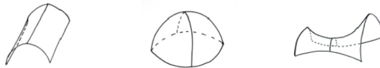
Figure1. Types of Shell [Single-curved, Double-curved (Synclastic and Anticlastic)].
