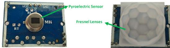
There are two important materials present in the sensor one is the pyroelectric crystal which can detect the heat signatures from a living organism (humans/animals) and the other is a Fresnel lenses which can widen the range of the sensor. Yes the white colour things is just a lense that is used to widen the range of the sensor, if you remove the lense you can find the Pyroelectric sensor inside it covered inside a protective metal casing as shown above.
