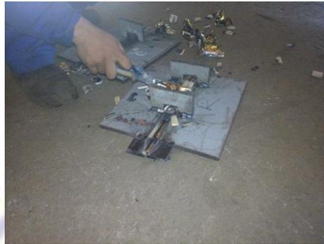
Gambar 4.6. Pelepasan Backing Ceramic
