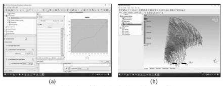
Fig.2. Setting of Crank Angle (a) and Contour (b)
