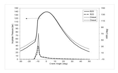
Fig.3. In cylinder Pressure and Heat Release rate
