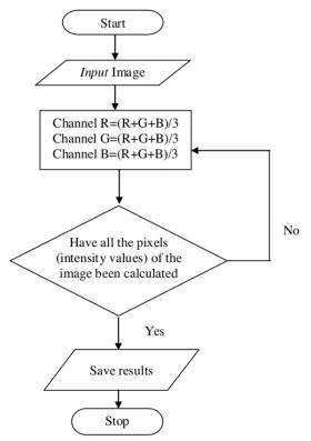
Figure 1. Flowchart of Grayscale Process
