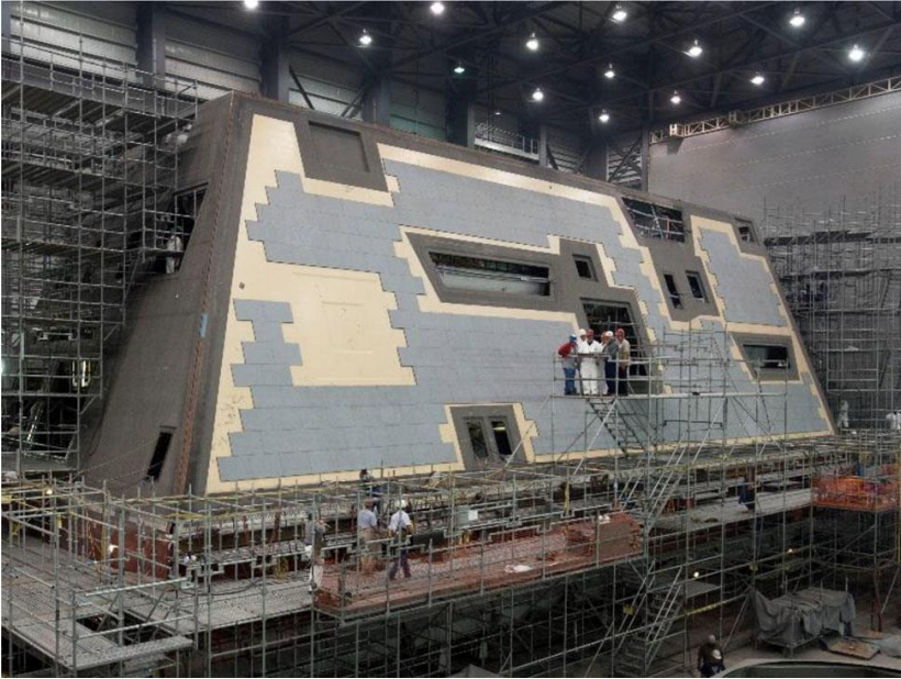
Gambar 4. Deckhouse kapal Zumwalt class destroyer selama proses konstruksi (Sumber: https://newsroom.huntingtoningalls.com ).
