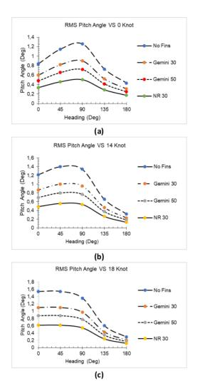
Figure 6. RMS Pitch angle at 0 (a), 14 (b) and 18 knots (c)
