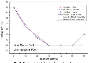
Fig. 7. Flash point of biodiesel based on days
