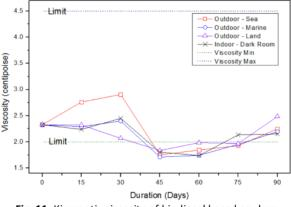
Fig. 11. Kinematic viscosity of biodiesel based on days
