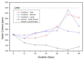
Fig. 12. Water content of biodiesel based on days
