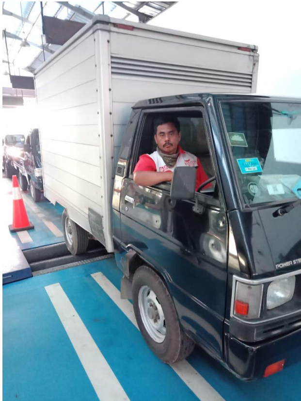
Lampiran 1 Gambar proses pengujian static brake test
