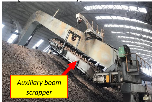
Gambar 2. 9 Auxiliary boom scrapper (Sumber: Dokumen Peneliti)
