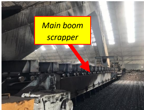
Gambar 2. 8 Main boom scrapper (Sumber: Dokumen Peneliti)
