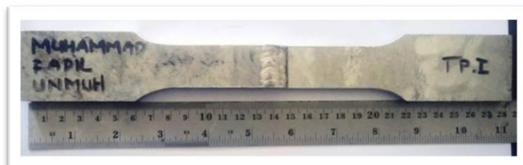
Gambar 3.19. *Test pieces tensile strength*
