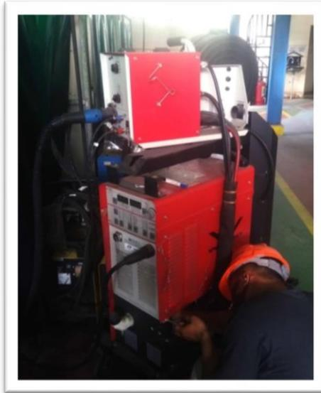
Gambar 3.9. Mesin Las GMAW (*Gas Metal Arc Welding*) Weiro WM350FA
