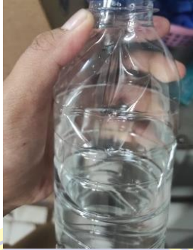
Gambar 4. 15 Defect Botol Peyok (Sumber: PT. UMSurya Bina Bangsa)
