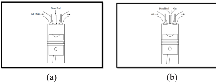
Gambar 3. Skema Port Injected (a) dan Directed (b) DDF [Ghazi A Karim, 2015]
