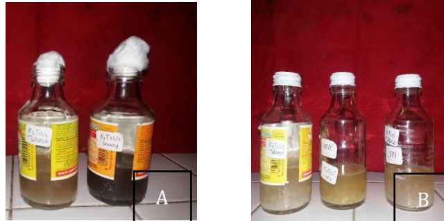
3 Figure 1. Color changes in the media exhibited by the bacterial isolates at 28°C after 14 days of incubation (A: High-Density Polyethylene Plastic; B: Low-Density Polyethylene Plastic)
