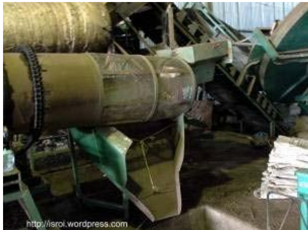
Gambar 20. Ayakan puter (rotary screener)
