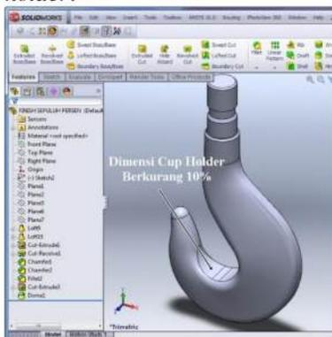
Gambar 14. Pemodelan 3D Hook Crane Cup Holder Berkurang 10%.
