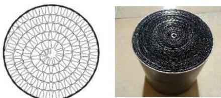
Fig. 5. *Chrome-coated copper (Cu+Cr) catalytic converter*. Diadaptasi dari (Warju et al., 2018)
