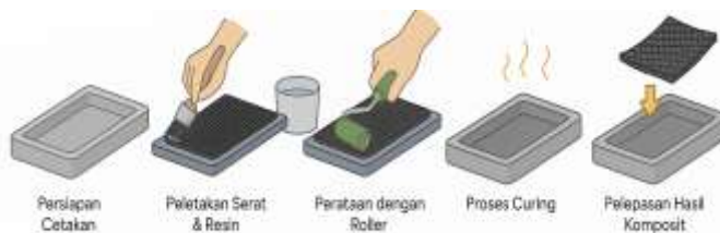
Gambar 2. 12 Proses Hand Lay Up (Sumber: Olahan Peneliti.)
