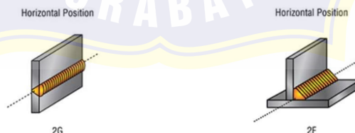
Gambar 2. 15 Posisi mendatar ( horizontal ) 2F / 2G (Miller,2021)
