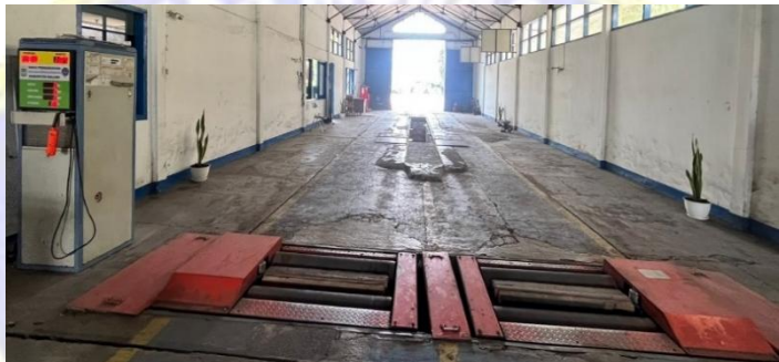
Gambar 3. 6 Alat Uji Berat ( Axle Load Tester )
