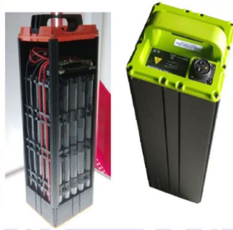
Gambar 2.14 Baterai Pack 20S4P 72V 20Ah
