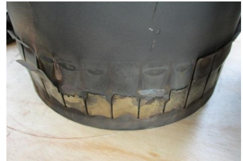
Figure 14. Hula Seal Damage to Combustion Liner Before MI CTG 101
