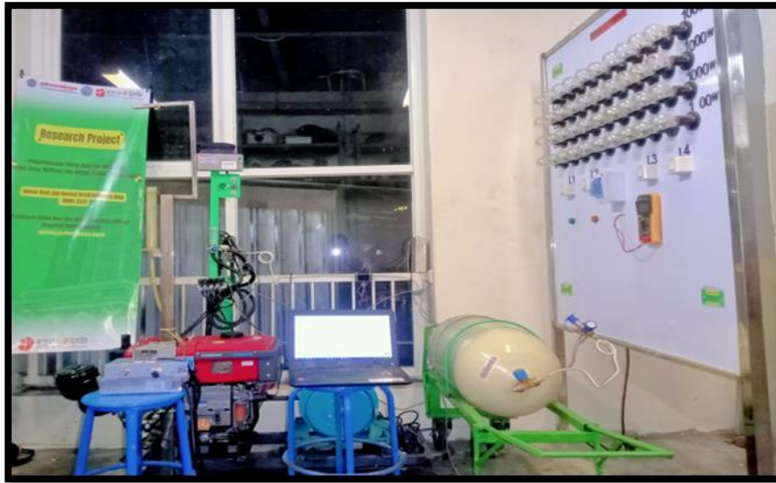
Figure 2. Laboratory-Scale Prototype of Natural Gas/Diesel Dual Fuel System with HHO Injection
