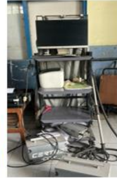
Figure 4. Tools of equipment \lambda , CO, CO 2 , O 2 , HC Merk : Certus Type : VMD400
