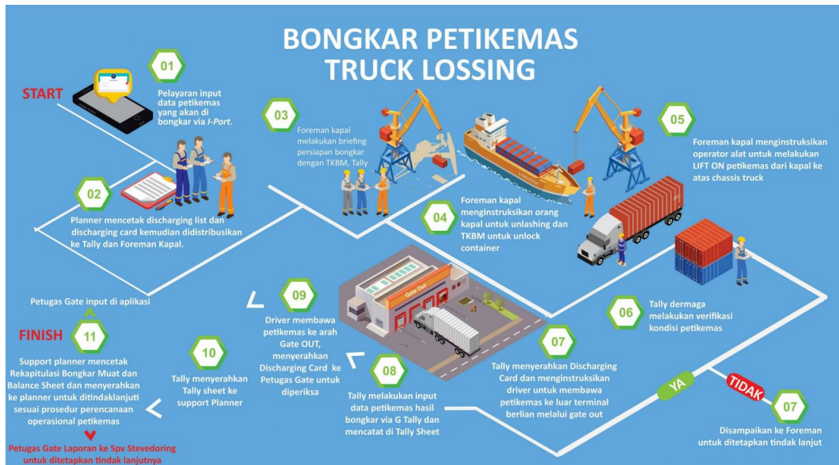
Gambar 2. 13 Alur Bongkar Peti Kemas Truck Lossing
