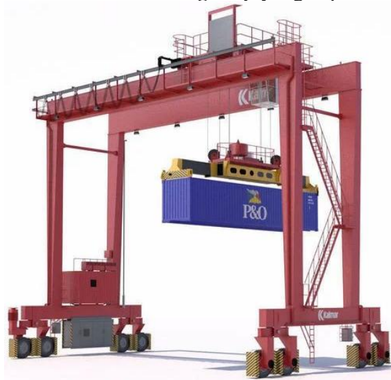
Gambar 2.5 Rubber Tyred Gantry
