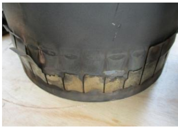
Figure 14. Hula Seal Damage to Combustion Liner Before MI CTG 101
