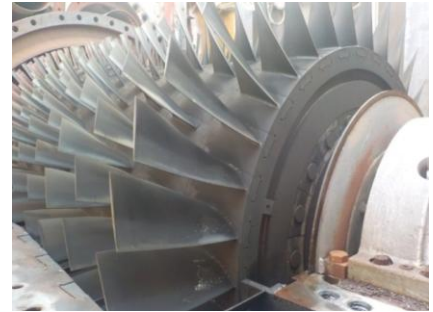
Figure 10. Fouling conditions on the Compressor Rotor Blade before MI CTG 101
