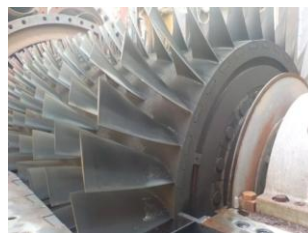
Figure 10. Fouling conditions on the Compressor Rotor Blade before MI CTG 101
