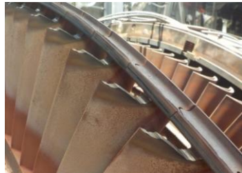
Figure 11. Turbine Stage 2 Bucket Damage before MI CTG 101
