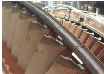
Figure 11. Turbine Stage 2 Bucket Damage before MI CTG 101
