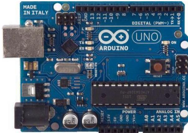
Gambar 2.2 *Board* Arduino Uno
