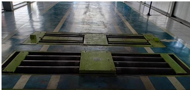
**Gambar 3 4** *Speedometer Tester*
