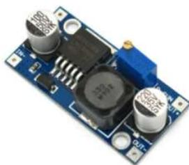
Gambar 2.17 Buck Converter LM2596
