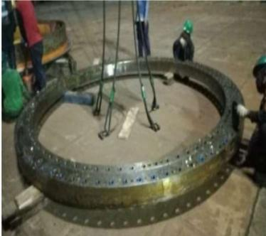
Gambar 2. Main Rotating Bearing (MRB)
