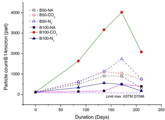
Fig. 7 - Particle count 14 μm of biodiesel gas blanket
