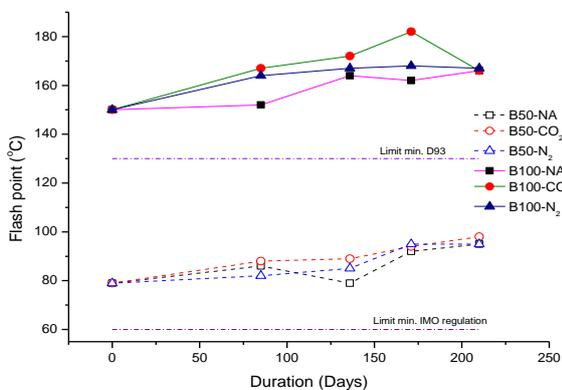
**Fig. 2 - Flash point biodiesel gas blanket**
