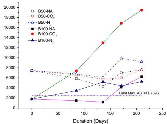
Fig. 5 - Particle count 4 μm of biodiesel gas blanket
