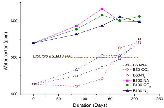
Fig. 9 - Water content of biodiesel gas blanket
