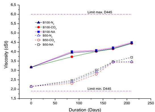
**Fig. 3 - Kinematic viscosity of biodiesel gas blanket**
