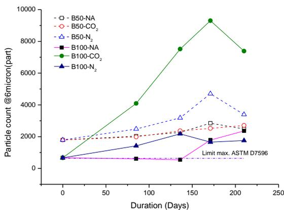
Fig. 6 - Particle count 6 μm of biodiesel gas blanket
