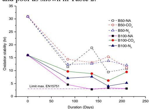
Fig. 11 - Oxidation stability of biodiesel blanket
