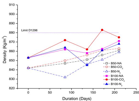
Fig. 4 - Density of biodiesel gas blanket
