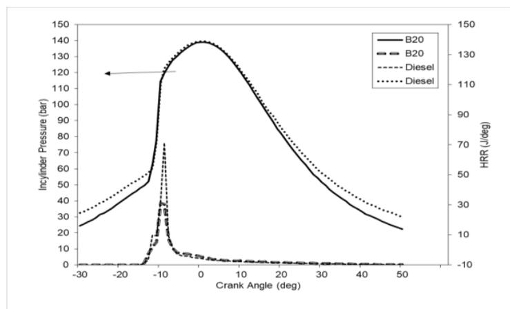
Fig.3. In cylinder Pressure and Heat Release rate
