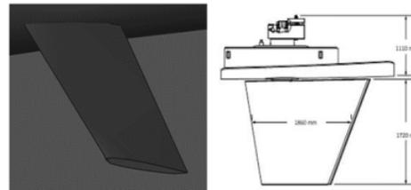
Figure 2. Gemini 30 Fins modeling and dimensions
