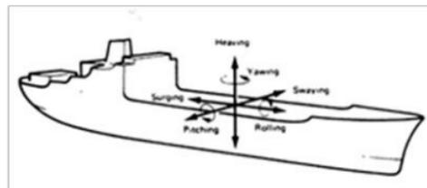
Figure 1. Six degrees of movement
