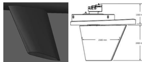
Figure 3. Gemini 50 Fins modeling and dimensions
