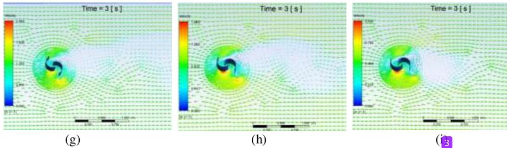
Figure 13. Vektor plots for SHT blades at three different velocity inlet: (g)  $V: 1.3 \text{ m/s}$ , (h)  $V: 0.9 \text{ m/s}$ , (i)  $V: 0.5 \text{ m/s}$ .
