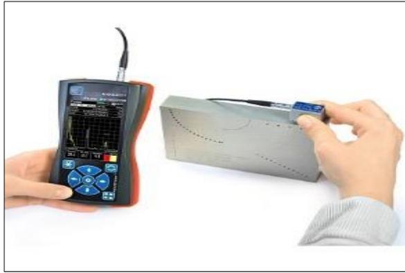
Gambar 2.8. Alat *Ultrasonic Flaw Detector*
